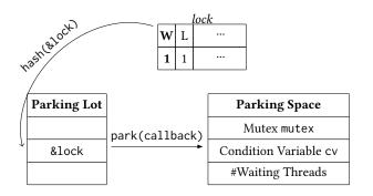
**Figure 5: Parking Lot** – All waiting threads park themselves in the Parking Lot (global hash table) until the callback-condition is fulfilled. The suitable Parking Space is determined using the lock's address.
