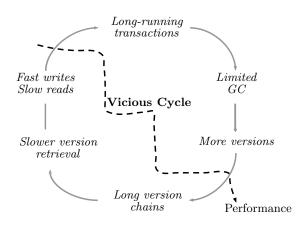
Figure 1: **MVCC's vicious cycle of garbage** – Old versions cannot be garbage collected as long as there are long-running transactions that have to retrieve them
